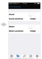
"Tap Arrow button" → "Tap Alarm Notification" → "Enter the admin user name and password" >> "Select the trigger source for alarm notification"→ "Tap Update"
