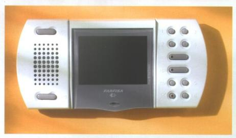
New Echos range models have been conceived in colour version, with 3.5" LCD screen, adjustable on horizontal axis for the best adaptability to avoid any light reflexes. Also this feature is very exploitable to properly adjust screen position according to the user tallness. Main feature of this monitor is its hand-free and open voice operation, no handset is
