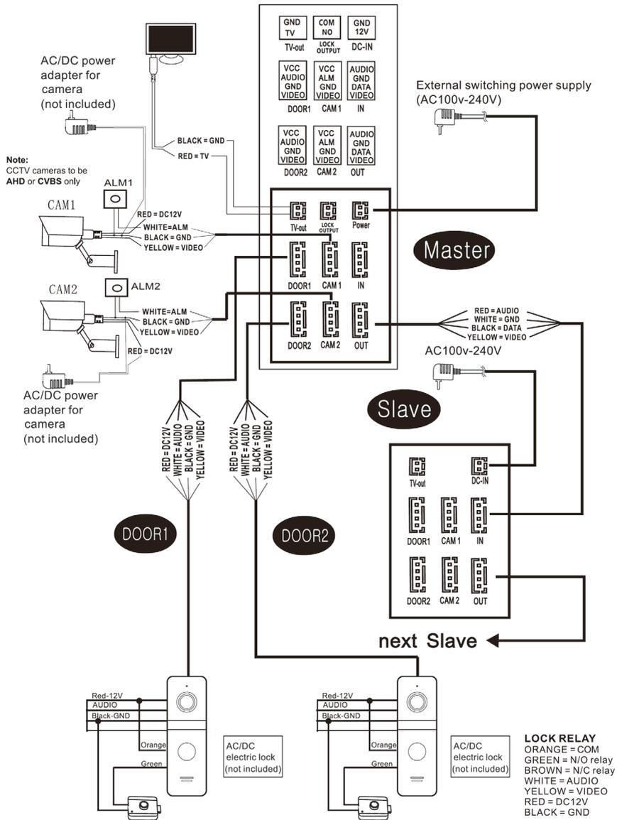
\*The first monitor is the MASTER monitor and ID must be set as Device 01. All other monitors are SLAVES and must be set as Device 02 to 06. To program the device ID go to MODE section.\*
