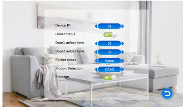
**[Device\_ID]:** Indoor monitor ID number 01/02/03/04/05/06 options, “01” means master monitor, “02-06” means slave monitor.
