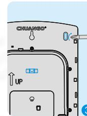
Hinge the front cover locating tabs over the top edge of the back plate and carefully push the base of the siren cover into place. Secure the siren cover in place by refitting the fixing screw in the bottom edge of the cover.
