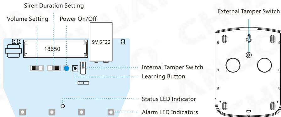
**Note:** The status LED will flash once every 5 seconds in arm status. It will not flash when in disarm status. The siren will sound immediately if the tamper switch is triggered.
