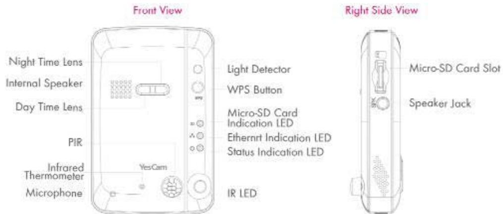
Figure 2-1: Major components in the front panel
