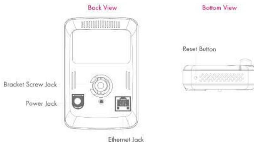
Figure 2-2: Major components in the back panel
